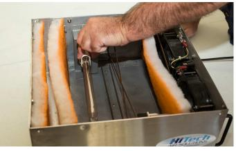
4. Install by holding on the base only. Lean bulb over in the direction of the safety latch on the socket, insert the bulb and then straighten bulb as it inserts into the bulb socket.
