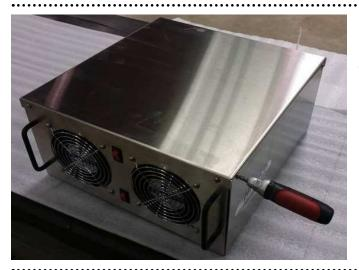
2. Remove the eight (8) phillips head screws that secures on the top of the unit.
