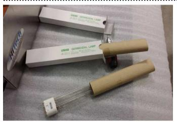
3. Remove bulbs from packing and install.
